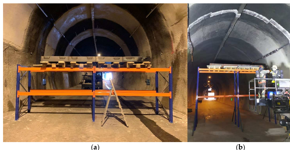
Figure 3. Fuel pan platform configurations: (a) arrangement at 2.1 m elevation; (b) arrangement at 4.1 m elevation.
